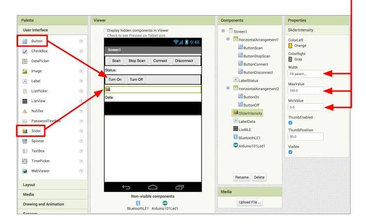
Drag a **Label** from the User Interface drawer in the Palette window and drop it between **SliderIntensity** and **ListBLE**.
